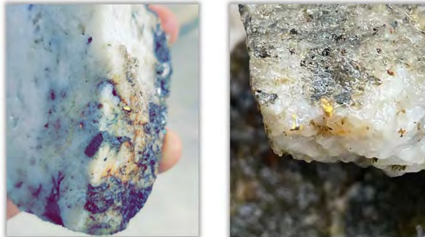
Figure 9.8: Photos of visible gold from Golden Glove Prospect (Source: Labrador Gold Corp., Assessment Report 2021)
